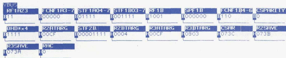
Fig. 3. Each CPU or memory board is designed such that most of its flip-flops, flags, and registers form a large circular shift register or "shift string." This is a diagram of a shift string and the corresponding console display. The string is broken up into fields determined by the designer.
